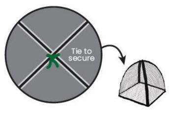
Secure cover to poles at roof pitch using ties attached to the inside of the cover.
